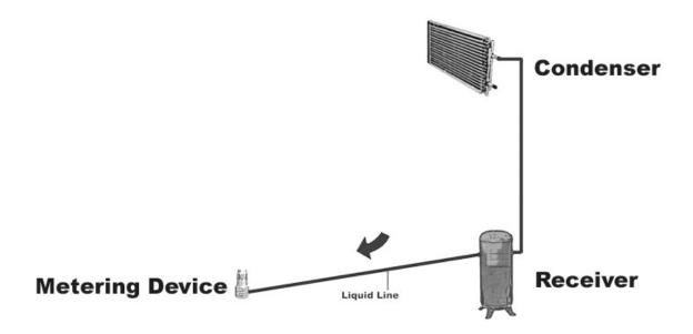
Systems using thermal expansion valves may have a receiver/tank on the outlet side of the condenser, designed to hold liquid refrigerant. When leaving the condenser directly or the receiver, the refrigerant remains a high pressure/high temperature liquid until it goes to the metering device. The line between the condenser and the metering device is also referred to as the **liquid line**.
