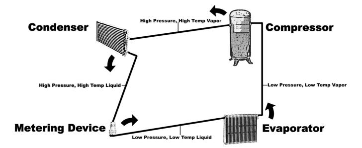
The **refrigeration process** is essentially the transfer of heat from one place to another. For example, in an air conditioning unit, the heat is removed from inside the building and is deposited outside the building. The vapor-compression refrigeration cycle is a repeating cycle consisting of four main components: the evaporator, compressor, condenser and metering device.
